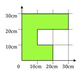
A flat piece of metal of uniform density has the shape and dimensions shown here. The center of mass for the piece of metal is located at:
