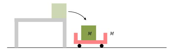
At the location where the box would have struck the floor, now a small cart of mass M = 3.0 kg and negligible height is placed. The box lands in the cart and sticks to the cart in a perfectly inelastic collision.
