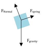
b. The force of gravity acting down the ramp ( $F_{\text{g-parallel}}$ ) pulls down on the mass until the force of the spring is pushing up with an equal amount of force. (See diagram next page.)
