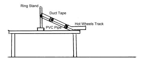
Use the materials provided to build a ramp on your table that will be used to roll a steel ball down. The top of the ramp should be at least 0.4m above the surface of your table. The lower section of the ramp must be horizontal so that the ball bearing is moving only horizontally when it becomes a projectile.
