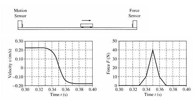
**2000B1.** A motion sensor and a force sensor record the motion of a cart along a track, as shown above. The cart is given a push so that it moves toward the force sensor and then collides with it. The two sensors record the values shown in the following graphs.
