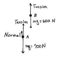
For a free body diagram that includes any one of the three forces on Student A (weight, normal, or tension)
